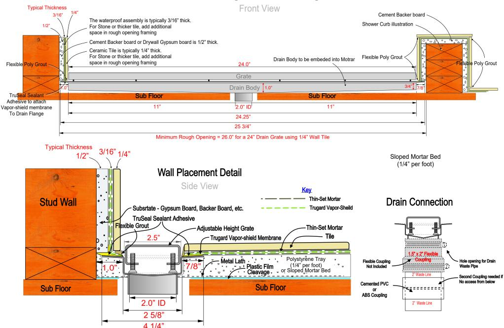
Note: To determine the framing rough opening size, add one inch to the length or width of the drain body, if a one quarter inch thick tile is being used. If the tile or stone is thicker than the 1/4" and the additional thickness of the tile to the 1 inch distance normally used to determine the rough opening size. So for example, for the rough opening for a 24 inch linear drain, the rough opening would need to be 26 inches, when 1/4" tile is being used.
