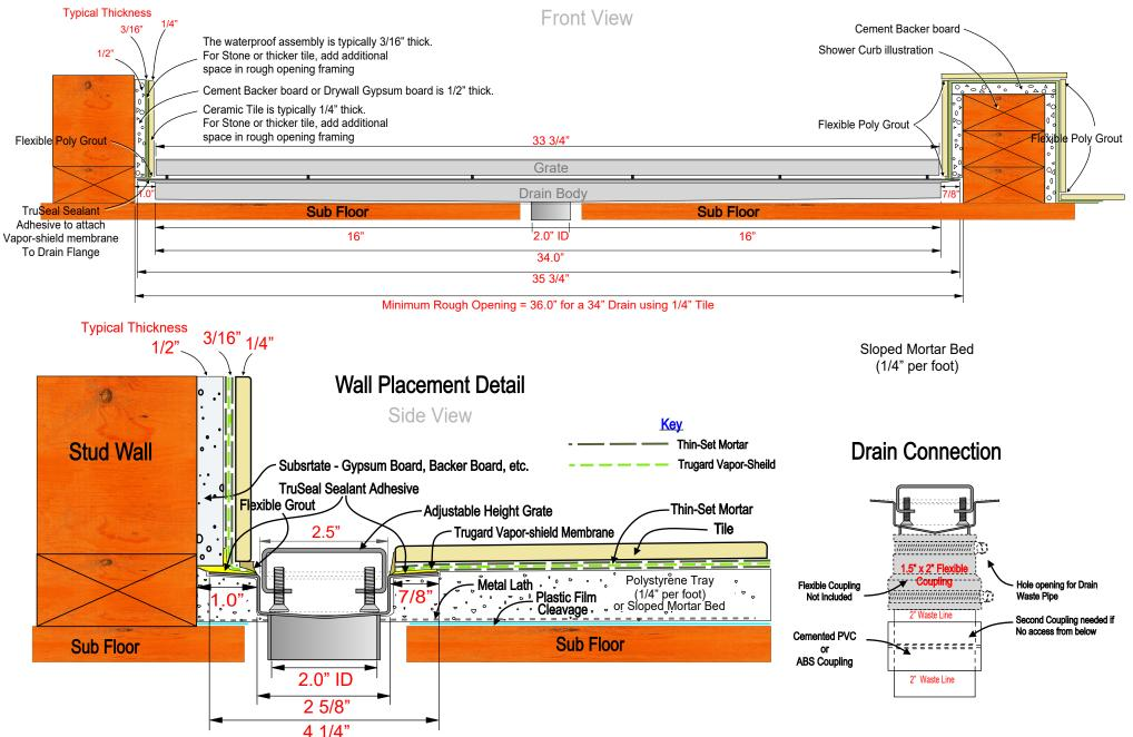
Note: To determine the framing rough opening size, add one inch to the length or width of the drain body, if a one quarter inch thick tile is being used. If the tile or stone is thicker than the 1/4" and the additional thickness of the tile to the 1 inch distance normally used to determine the rough opening size. So for example, for the rough opening for a 34 inch linear drain, the rough opening would need to be 36 inches, when 1/4" tile is being used.
