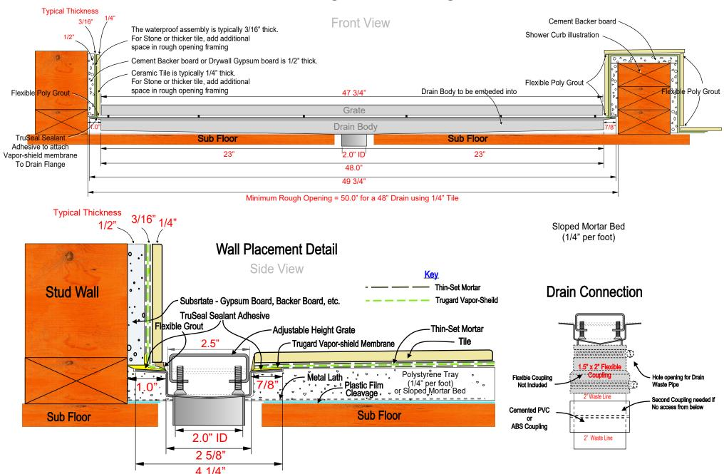
Note: To determine the framing rough opening size, add one inch to the length or width of the drain body, if a one quarter inch thick tile is being used. If the tile or stone is thicker than the 1/4" and the additional thickness of the tile to the 1 inch distance normally used to determine the rough opening size. So for example, for the rough opening for a 48 inch linear drain, the rough opening would need to be 50 inches, when 1/4" tile is being used.
